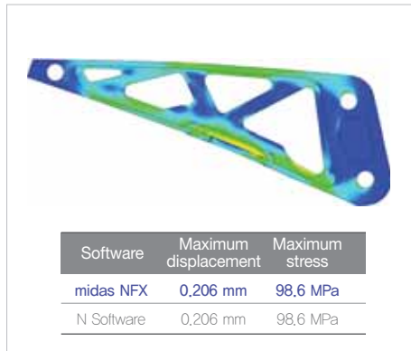
Linear static analysis (solid element, rigid link, concentrated load)
