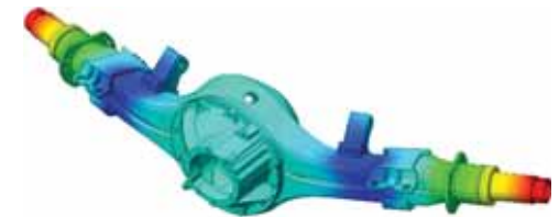
Modal analysis of an automobile axle (7th mode, Free-Free condition)
