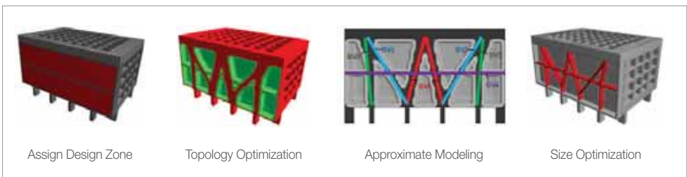
Size optimal design using topology optimization
