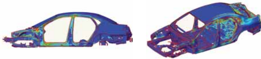
Dynamic analysis of a car body
