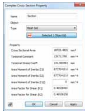
Complex Cross-Section Property window
