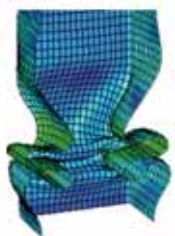
Nonlinear contact analysis of steel frame
